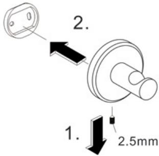
1. Loosen the set screw on the accessory and remove the backing plate. Position the accessory against the wall and mark outline with pencil.
