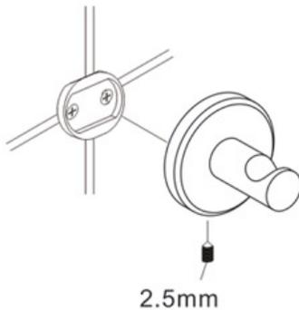
4. Slide the accessory onto the backing plate and tighten the set screw using Allen Key provided.
