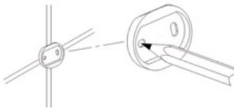
2. Position the backing plate flat side down on the wall and mark holes with pencil.
