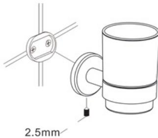
4. Slide the accessory onto the backing plate and tighten the set screw using Allen Key provided.
