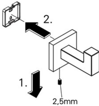
1. Loosen the set screw on the accessory and remove the backing plate. Position the accessory against the wall and mark outline with pencil.
