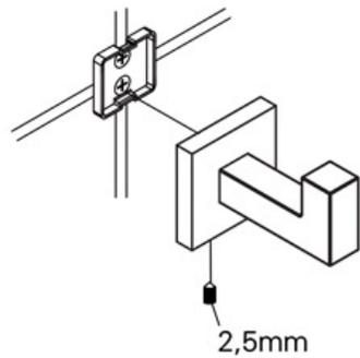
4. Slide the accessory onto the backing plate and tighten the set screw using Allen Key provided.
