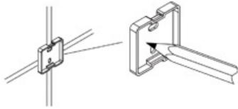
2. Position the backing plate flat side down on the wall and mark holes with pencil.
