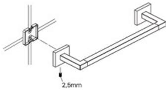
4. Slide the accessory onto the backing plate and tighten the set screw using Allen Key provided.
