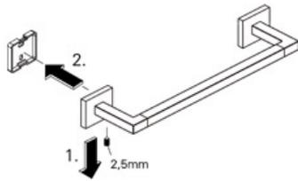
1. Loosen the set screw on the accessory and remove the backing plate. Position the accessory against the wall and mark outline with pencil.
