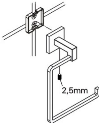
4. Slide the accessory onto the backing plate and tighten the set screw using Allen Key provided.
