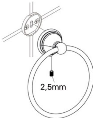
4. Slide the accessory onto the backing plate and tighten the set screw using Allen Key provided.
