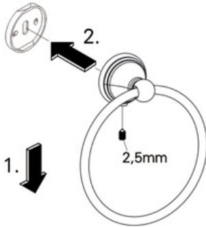
1. Loosen the set screw on the accessory and remove the backing plate. Position the accessory against the wall and mark outline with pencil.
