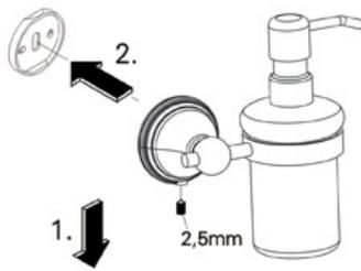
1. Loosen the set screw on the accessory and remove the backing plate. Position the accessory against the wall and mark outline with pencil.
