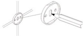
2. Position the backing plate flat side down on the wall and mark holes with pencil.
