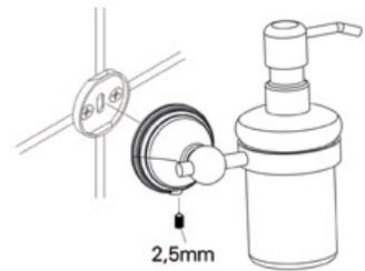
4. Slide the accessory onto the backing plate and tighten the set screw using Allen Key provided.
