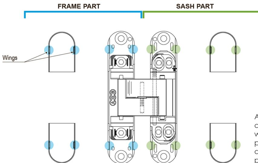
Apply the covers paying attention to the lateral wings. They have to be plugged into the dedicated grooves present in the hinge.
