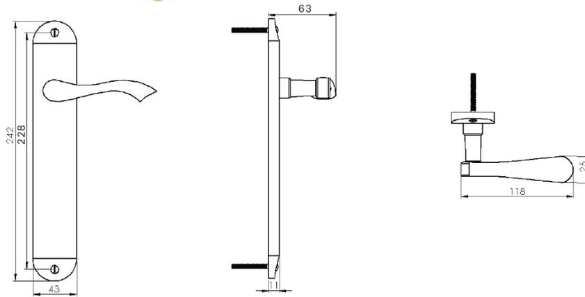
This latch handle is suitable for use with most U.K. tubular latches.
