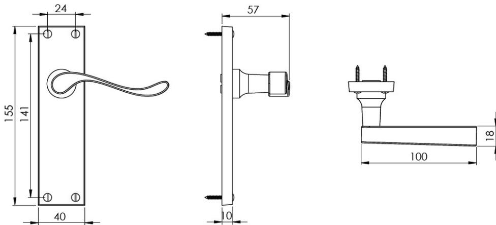
This latch handle is suitable for use with most U.K. tubular latches.
