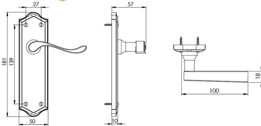
This latch handle is suitable for use with most U.K. tubular latches.
