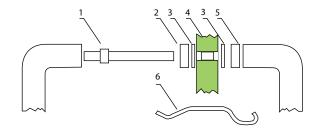
For use on timber & glass doors, from 12mm to 55mm.
